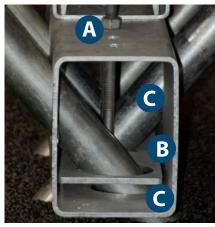
**8**. Ensure the pipe can easily slide through the side driving hole. **Important Note:** If pipe does not easily slide, loosen the nut (on top of beam), lowering the force plate.
