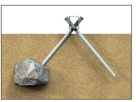
**2**. Cut the remaining portion of the pipe, above the Ground Frame beam, and cap. **Important Note:** Indicate the length of the pipe that was cut off in the driving log.
